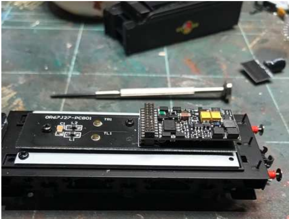
PCB screwed back down, and 21 sounder decoder plugged in above. Job done!
