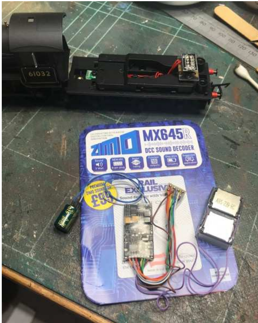
The Zimo decoder out of the packet as supplied by YouChoos, with my chosen speaker already wired.
